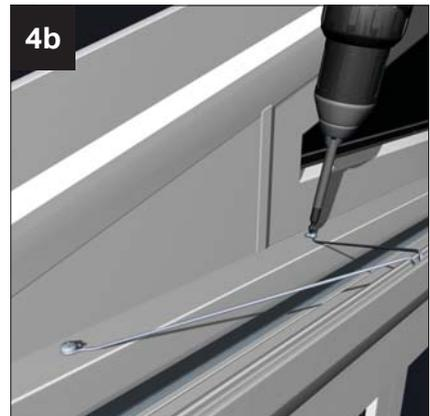
Fix wire ties at an angle as shown, ensure the Cornice is parallel to the frames/roof line.
